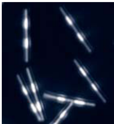
Optical microscope image of 300 nm x 6 micron barcoded particles (400 nm illumination). Bright segments correspond to Ag, and dark segments to Au.
