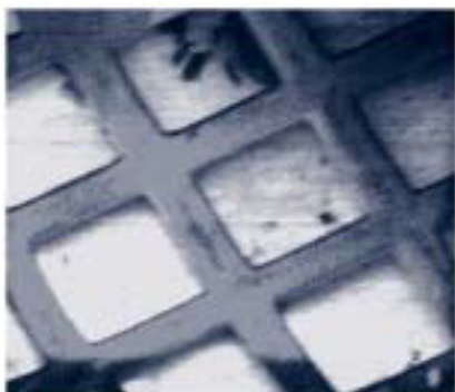
Copper grid over indium foil and a 100 micron field of view.
